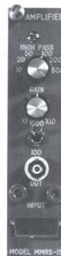
Close-up of MMRS-1S single-ended card showing 100-10,000 continuous gain control and 5-value Lo-cut filter selection. (This is only one example of possible configurations.)
